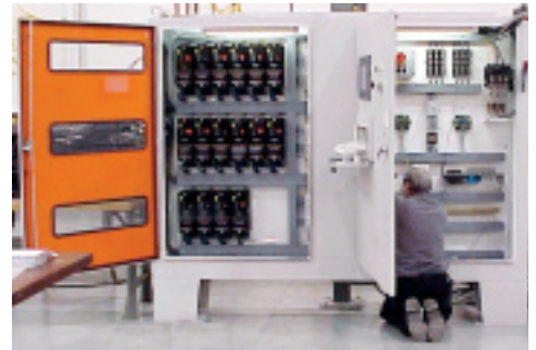
Custom CS7000 controls 16 Hi-Torque 177 Series spindles
