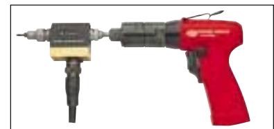
Calibration of pneumatic screwdrivers
