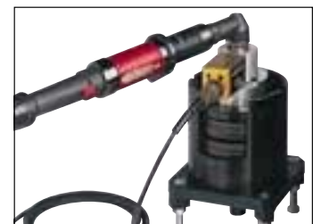
Calibration of controlled electric nutrunners.
