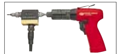
Calibration of pneumatic screwdrivers
