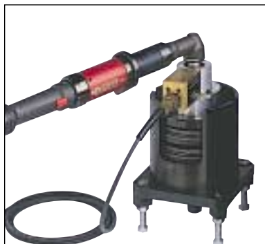
Calibration of controlled electric screwdrivers
