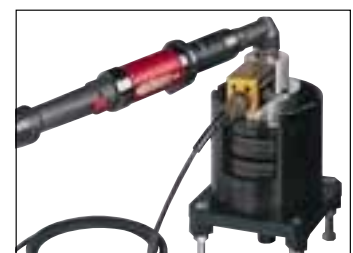
Calibration of controlled electric nutrunners.
